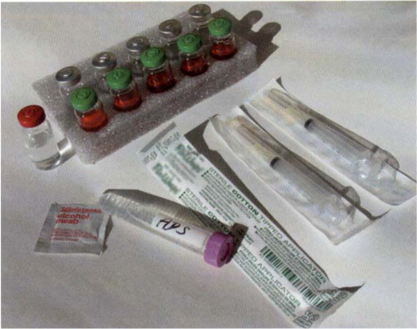
FIGURE 13 A typical commercially supplied bacteria culture test kit for APB and SRB.
