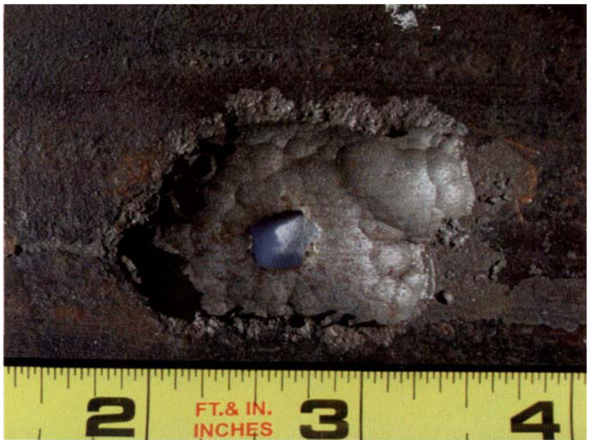
FIGURE 10 A corrosion pit that displays “cup-type hemispherical pits,” pits within pits, and faint striations that run parallel to the longitudinal axis of the pipe. These features alone are not diagnostic for MIC, rather, they are reported to occur as the result of under deposit acid attack of low carbon steels.
